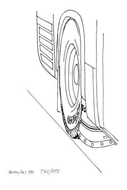
As noted in Figure 2, field trials do support the ability of this design to physically move a subject from the path of travel. This is helpful in instances where Bernoulli's principal is not a causal factor, as when transit buses turn into pedestrians or cyclists. In those instances, the guard must act much like the cowcatcher on a train and physically move the individual from the path of the rotating wheel.
